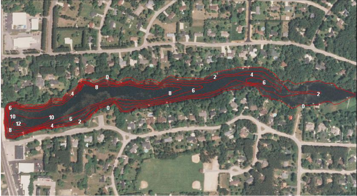
Figure 1. Map of Springville Pond showing depth contours. (Portage County Planning and Zoning
